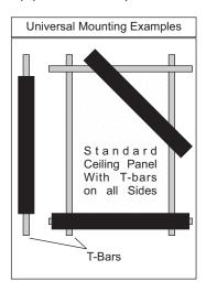
**STEP #2** - Affix the speaker to the metal T-Bar located in your ceiling. While supporting the speaker so it doesn't fall, screw Bracket-B into Bracket-A from the side and make sure the bracket is clamped over the T-Bar. When finished, the unit should look the illustration and photo below.
