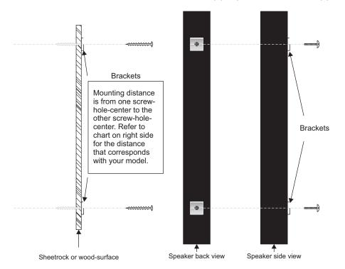
**STEP #2** - Mount speaker with brackets to installed wall brackets.
